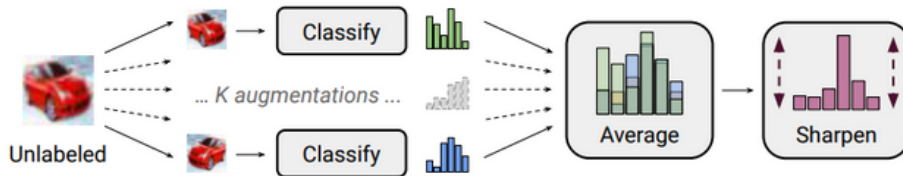
Figure 1: Diagram of the label guessing process used in MixMatch. Stochastic data augmentation is applied to an unlabeled image K times, and each augmented image is fed through the classifier. Then, the average of these K predictions is “sharpened” by adjusting the distribution’s temperature. See algorithm 1 for a full description.
